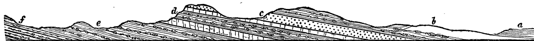
a. Lower Lias. b. Saliferous Marls, &c. c. Red Sandstone and Quartzose Conglomerate. d. Calcareous Conglomerate. e. Lower New Red Sandstone. f. Upper Coal Measures.
